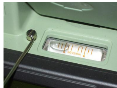
Tweak the adjusting screw with an adjusting pin with an adjusting pin
